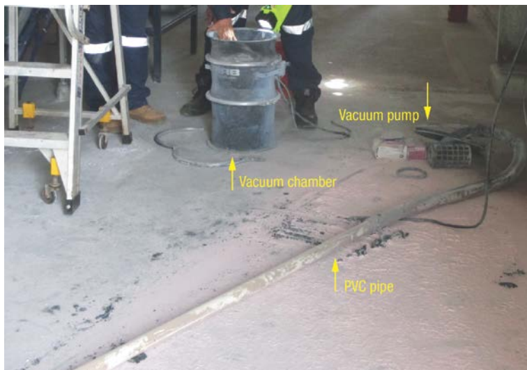
Damage to transfer system. Left. Vacuum pump chamber and pump, PVC transfer piping and evidence of spot fires on the floor. Right. Distortion of hopper caused by explosion.
