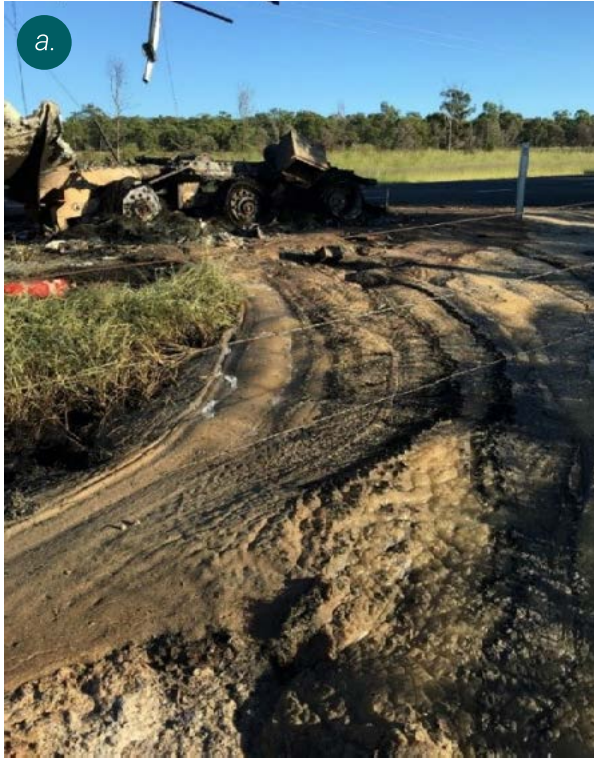
Figures 7.1 a and b Images of tanker trailer. This shows the flow of bulk unchanged ANE (i.e. had not undergone significant decomposition) that had escaped from the aluminium shell and was away from the tyre fire
