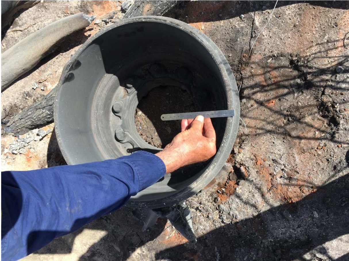
Figure 5.26 Brake drum weighing 60 kg located 97 m south-east of the epicentre of the blast
