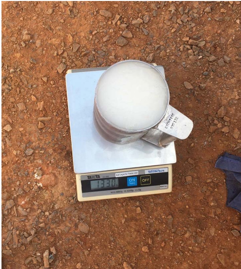
Figure A4.1 Density measurement of ANE from the tanker trailer that arrived at Gruyere mine site
