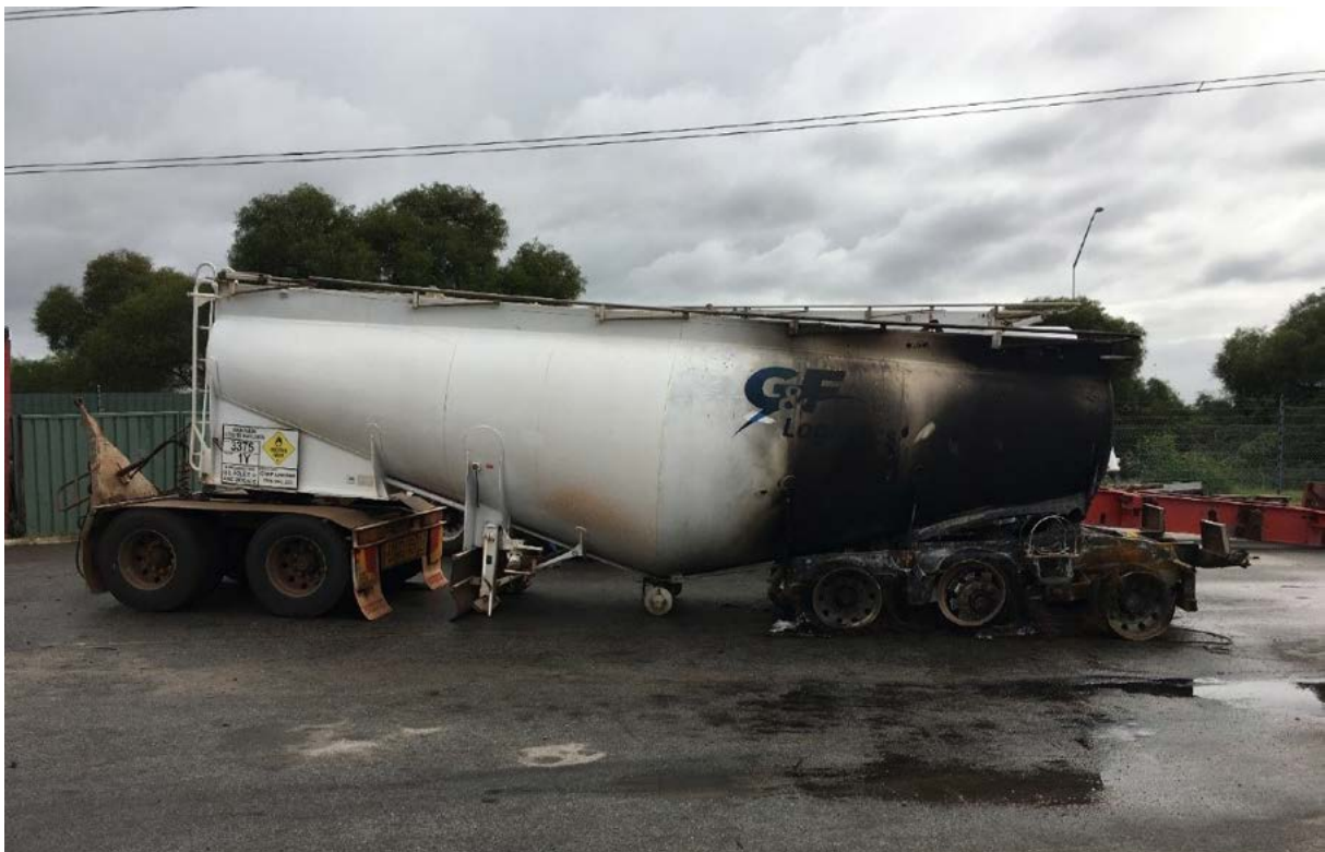
Figure 7.2 Tyre fire on the ANE tanker caused by wheel bearing failure
