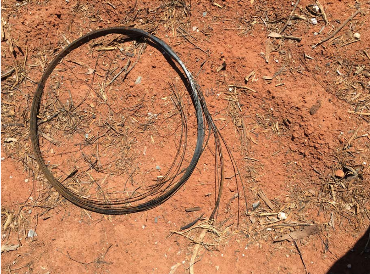
Figure 5.30 Inner steel radials used to reinforce tyre located within a 30 m distance from the epicentre of the explosion. Two spools were located within close proximity of one another
