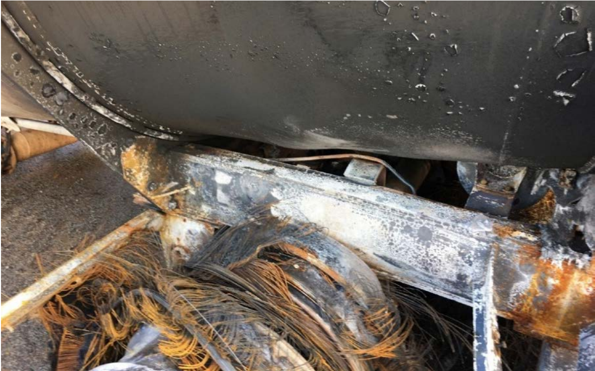
Figure 7.3 Tanker shell starting to buckle caused by the fire
