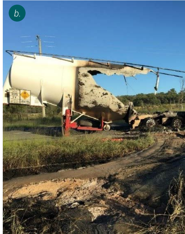
Figures 7.1 a and b Images of tanker trailer. This shows the flow of bulk unchanged ANE (i.e. had not undergone significant decomposition) that had escaped from the aluminium shell and was away from the tyre fire
