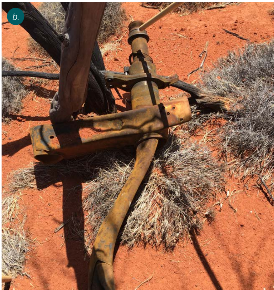
Figures 5.28 a and b Axle suspension arm from dolly (weighing in excess of 100 kg)
