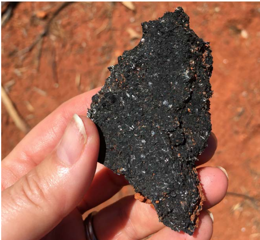
Figure 5.33 Tyre fragment that has been affected by fire located 66 m from epicentre in south-south-east direction
