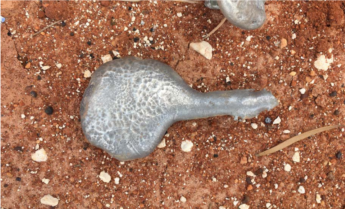
Figure 5.23 Image of molten aluminium pieces approximately 10 cm in length located 157 m west of the epicentre
