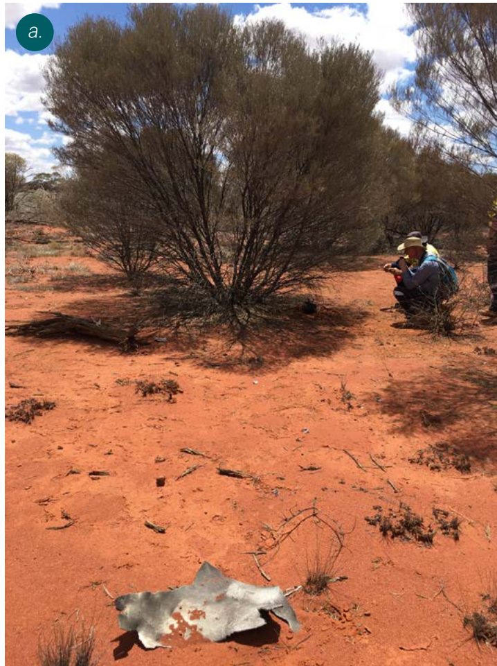
Figure 5.22a Aluminium fragment from intact section of tanker shell found to the south-south-east of the blast
