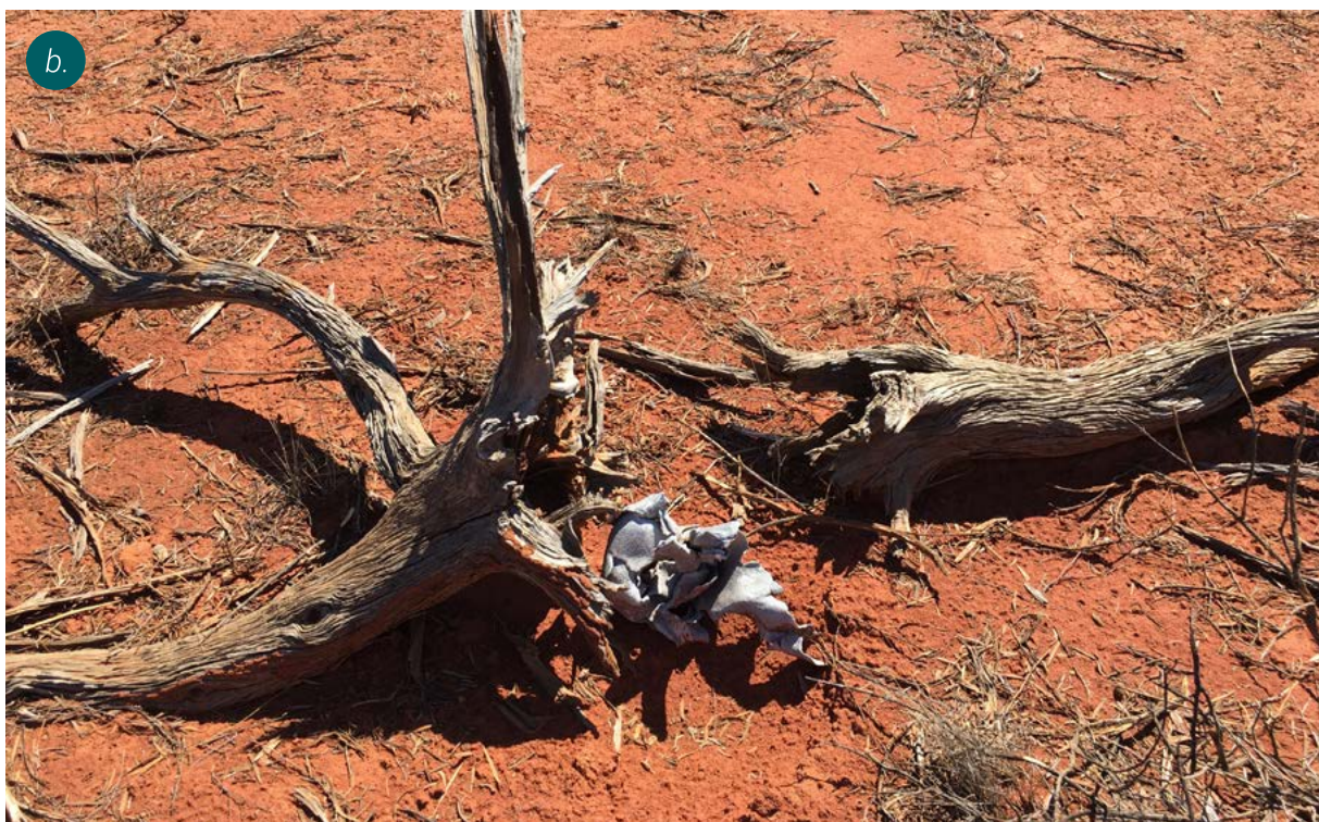
Figure 5.22b Aluminium shrapnel found at approximately 50 m to NW of the epicentre of the explosion
