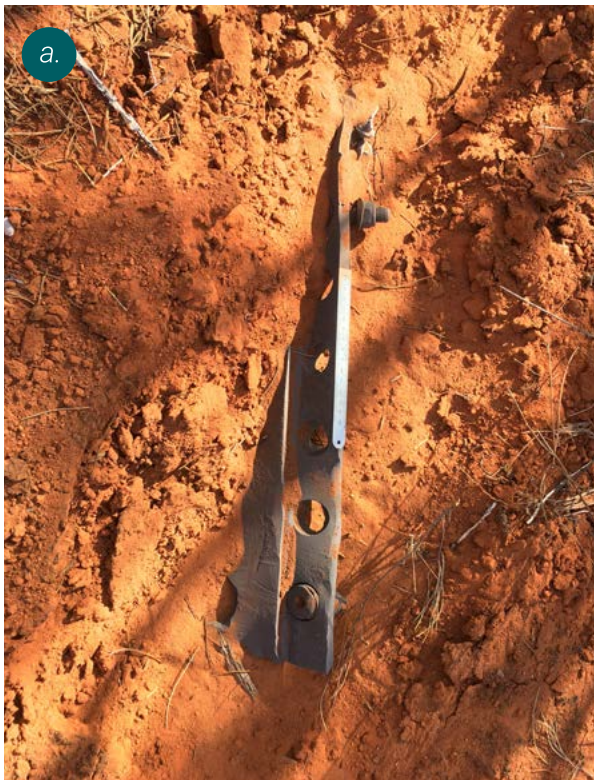
Figures 5.27 a and b Piece of dolly turntable, weighing 31 kg, found embedded within the ground at 672 m from the epicentre of the explosion
