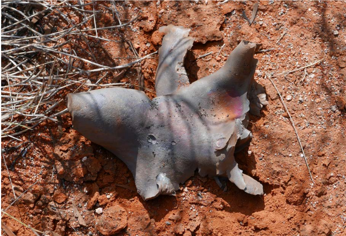
Figure 5.29 Steel piece of shrapnel (approximately 20 cm) with noticeable softening effects on the edges from the fire. Piece located at 304 m south-south-east of the epicentre of the explosion
