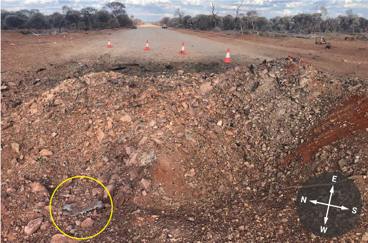
Figure 5.10 Image of crater looking east. Note solidified molten aluminium can be seen to the bottom left of the image (Credit: DFES)
