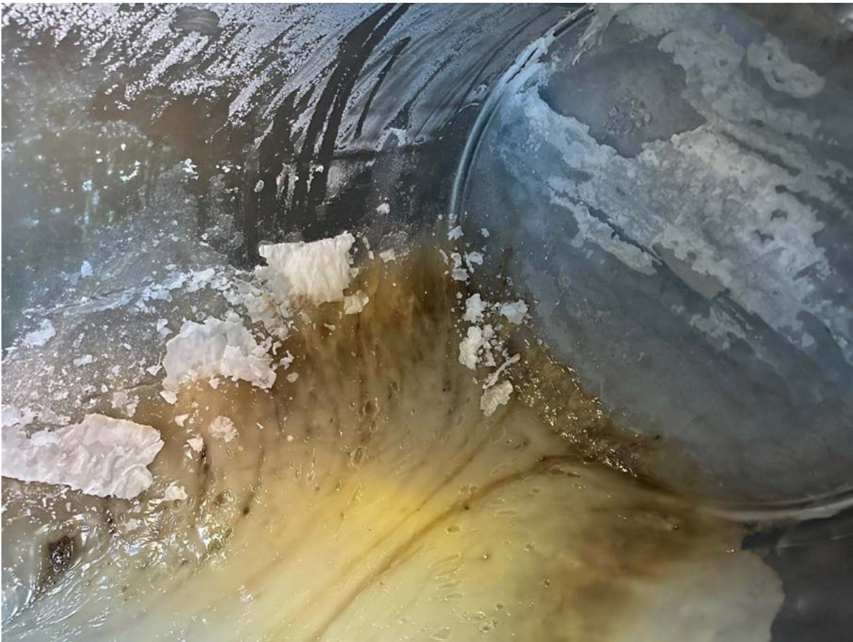
Figure 7.4 Inside walls of the tanker after the bulk of the ANE had been transferred. Solid AN formed on the sides where the fire impinged on the tanker. Some discolouration and possible separation of the product has occurred
