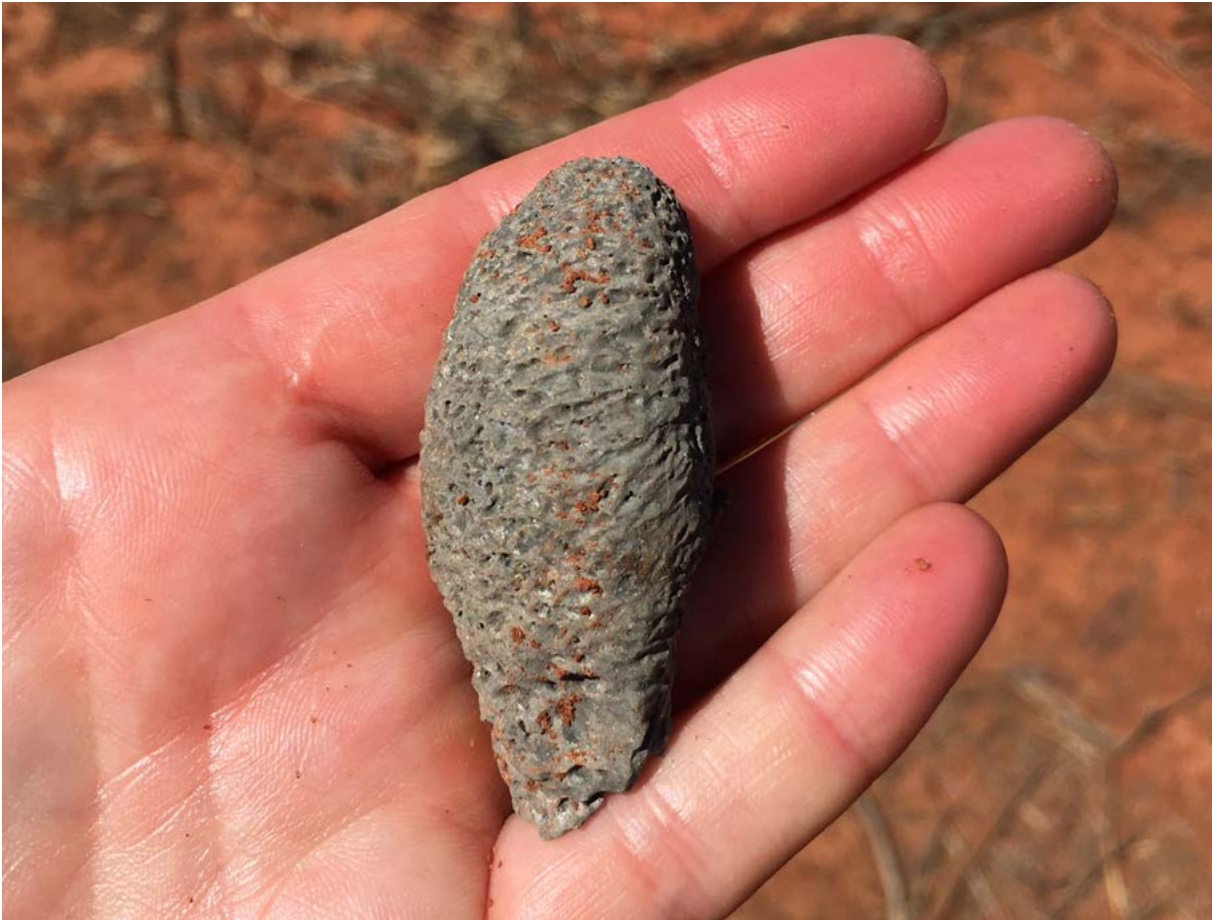
Figure 5.24 Another piece of solidified molten aluminium, pitted by the cooling on the ground and formed into a ball like structure
