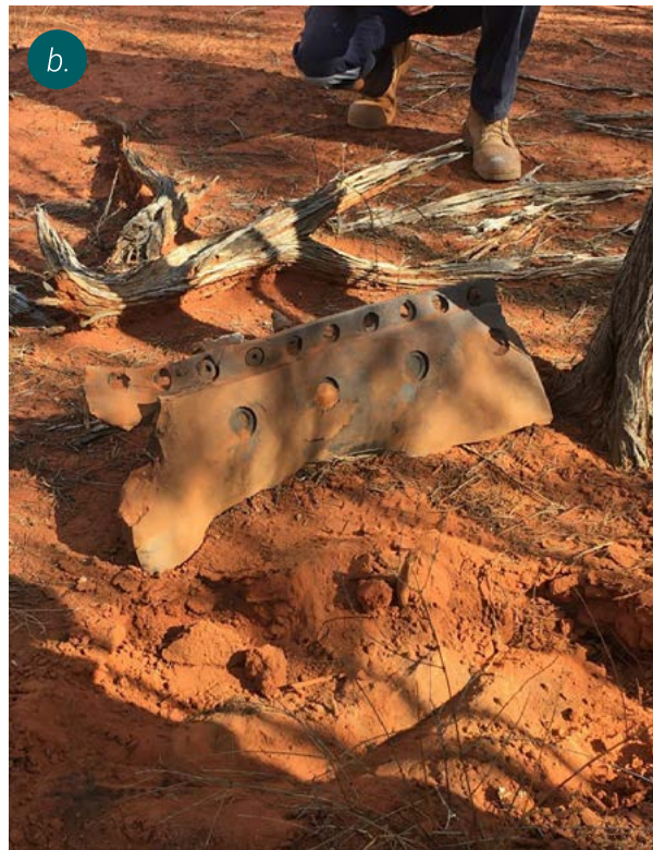
Figures 5.27 a and b Piece of dolly turntable, weighing 31 kg, found embedded within the ground at 672 m from the epicentre of the explosion
