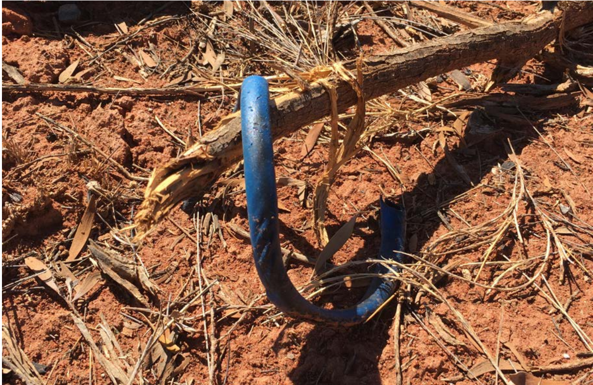
Figure 5.32 Air supply line cable located 61 m from the explosion site in an east-south-east direction. As it is relatively unscathed, it is thought that this was located towards the front of the dolly's draw bar and less subjected to fire
