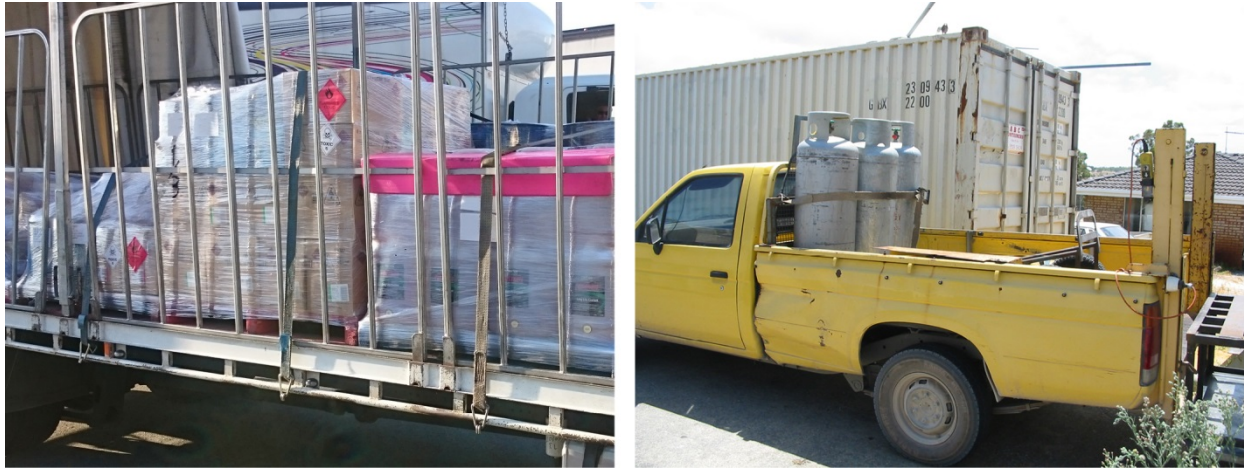
Restrained load examples. Left. Correctly restrained load with primary and secondary restraint (behind gates). Right: Incorrectly restrained load – rigid sides of insufficient height for load (e.g. load protruding more than 30 per cent above the rigid sides) and no gates.
