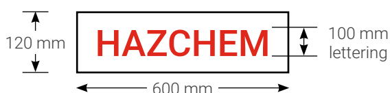
Figure 2 Sample outer warning placard
