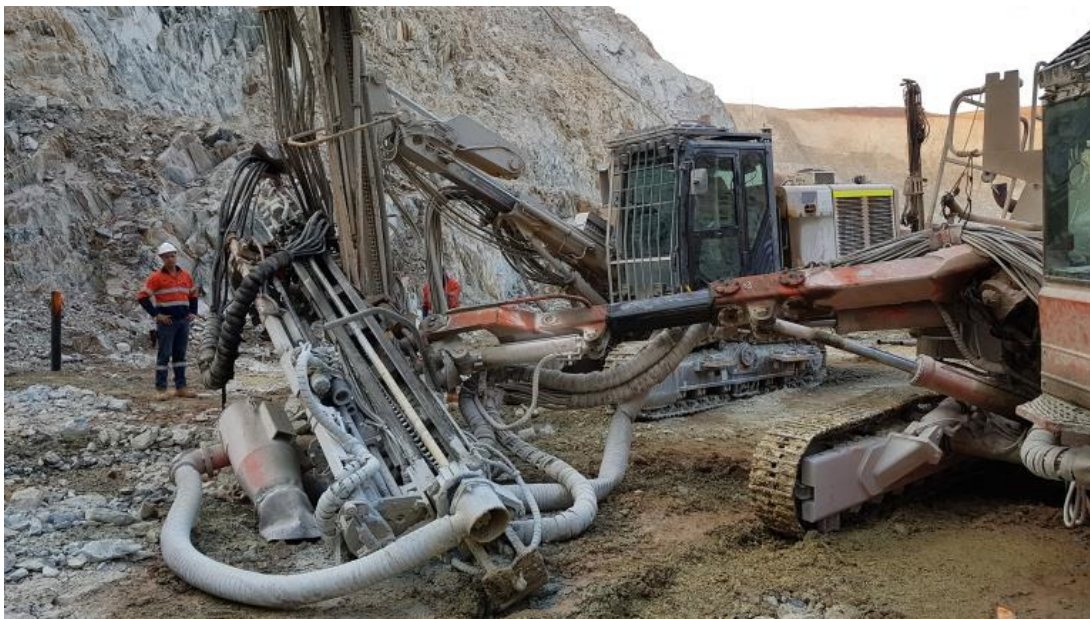
Failure of welds on drill rig's boom clevis plate (locating tab/plate) results in boom and mast falling.
