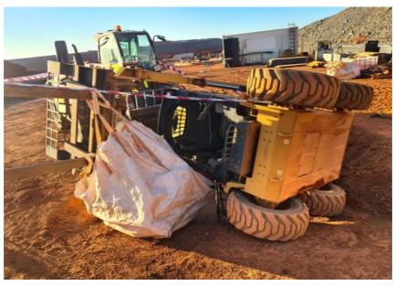
An operator was reversing a skid steer under the direction of a spotter when the back right side wheel went over an edge of shallow footing. With the momentum of reversing, the centre of gravity changed and skid steer tipped onto its side.
