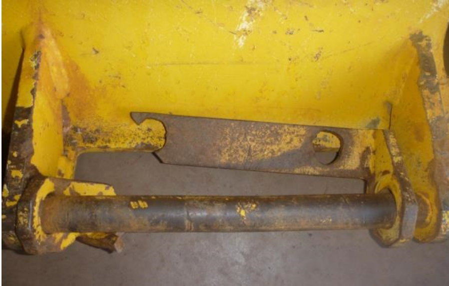
Damaged hinge on left-hand side of belly plate shown after cleaning.
