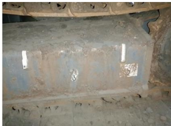
Left: Damaged step used as a lifting point with lifting point signage. Right: Rear track frame with failed step weld.
