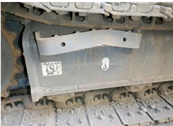
Left: Damaged step used as a lifting point with lifting point signage. Right: Rear track frame with failed step weld.
