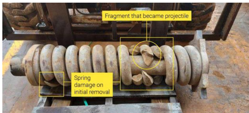
Recoil spring after removal from excavator prior to incident.
