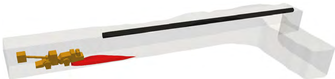
Figure 26: Regions where DPM concentrations are greater than 0.1 mg/m 3 in the mine region during charging activity
