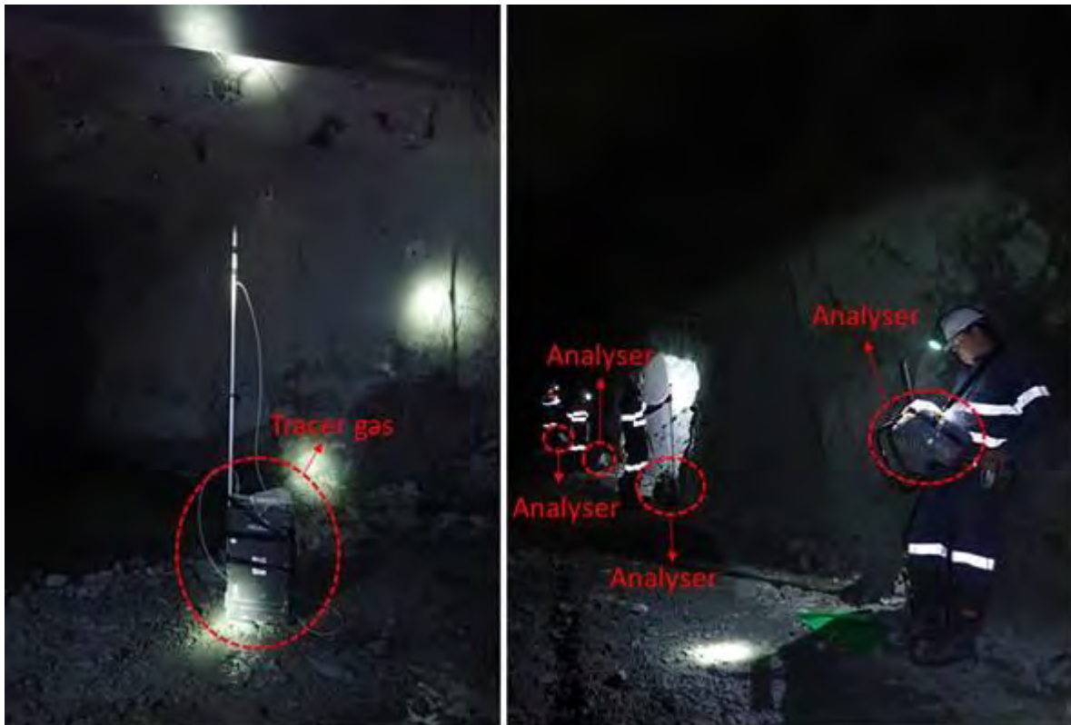
Figure 15: Tracer gas study during the Traverse exercise.
