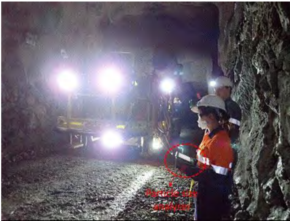
Figure 5: Particle size monitoring during the Charging activity.
