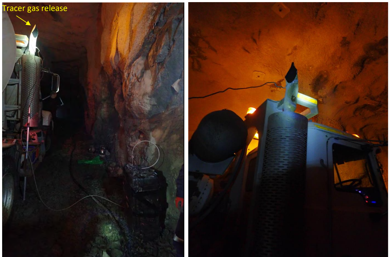
Figure 1: Tracer gas release into the Agi truck exhaust.
