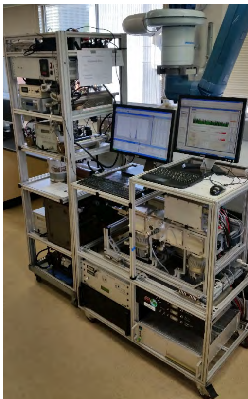
Figure 4 Image of the Aerosol Mass Spectrometer used in this project undergoing laboratory testing.
